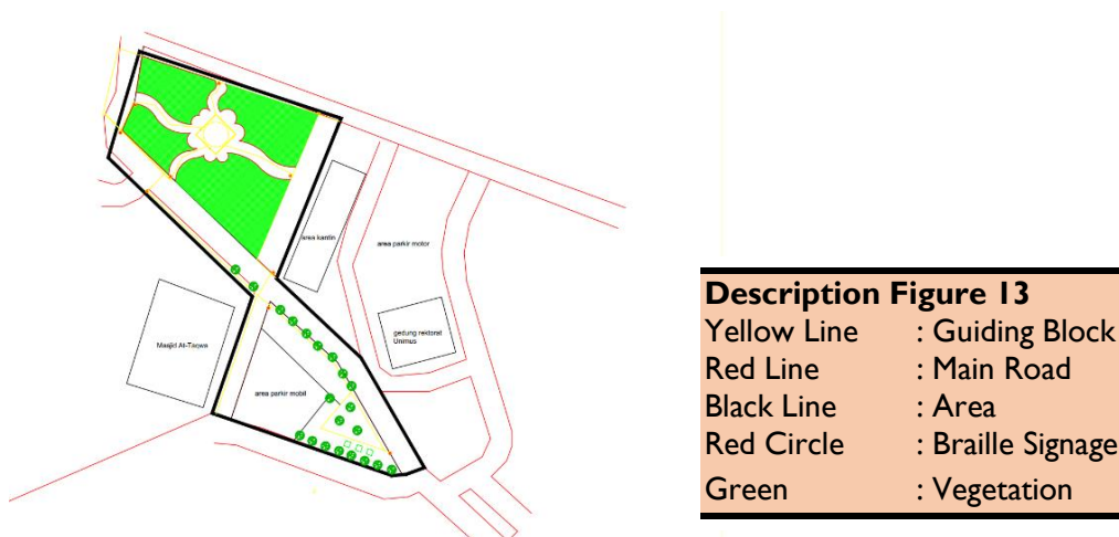
Figure 13. Plan for the Addition of Guiding Blocks and Braille Signage
